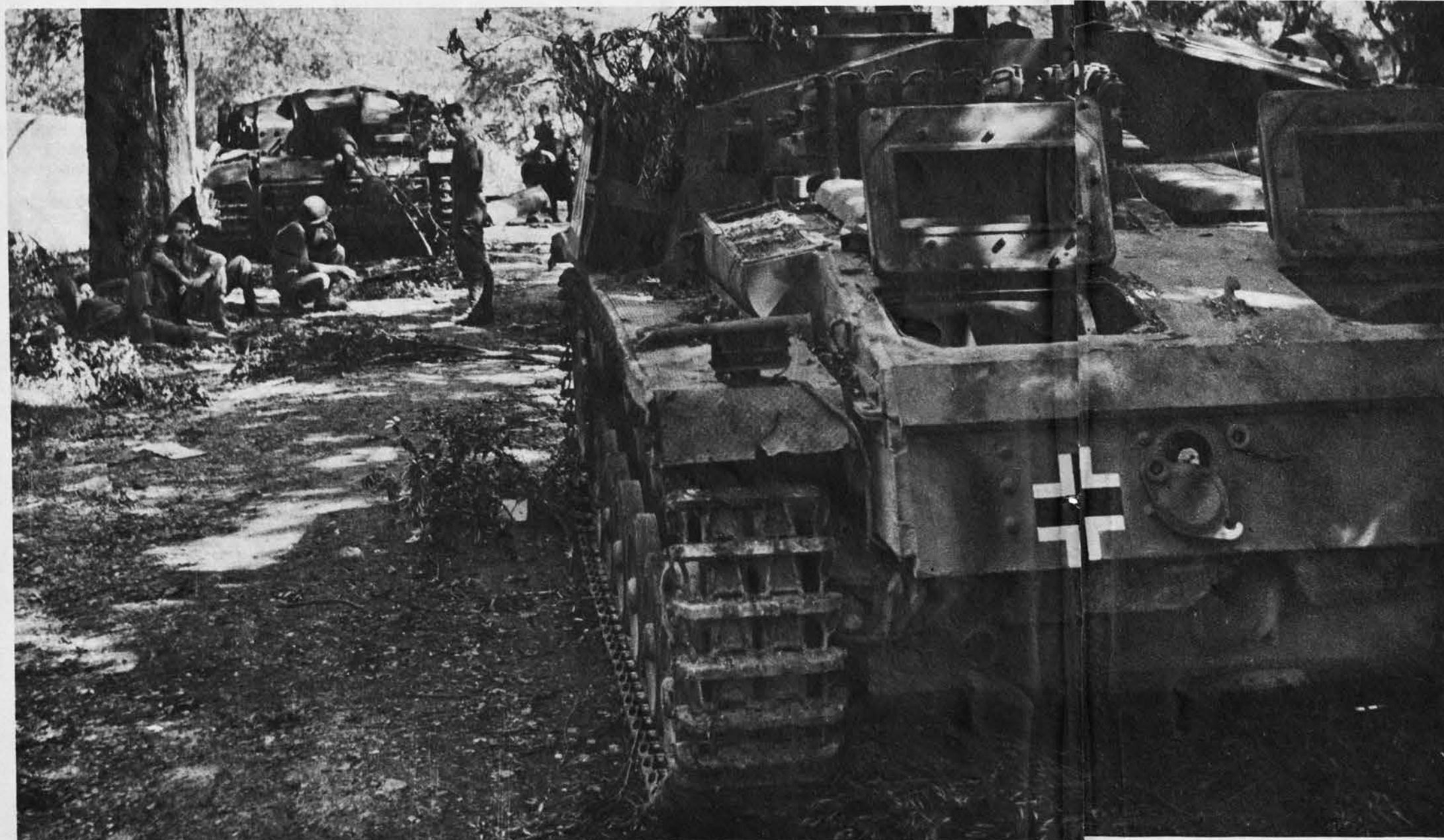
To pierce the Gustav Line , the Allied troops had to beat their way past many 75-mm. self-propelled assault guns on PzKw III chassis. These last-ditch defenders made the going tough
